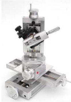
A four axis system to measure travel distance for medium-sized payloads.
