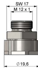
TM-TAS-CT Pivoted joint for CT sensors
