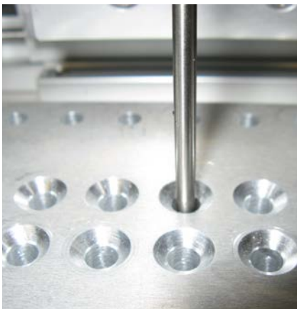
Diameter measurement in small bores with IFS2402/90 sensors
