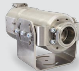
TM-J-TIM Cooling jacket (length 228mm, ø89mm) with adjustable mounting bracket TM-JAB-TIM; recommended high temperature cable TM-USBC5H-TIM (up to 240°C)
