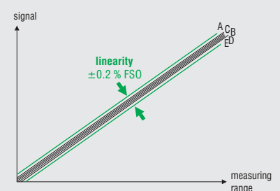
best practice: eddyNCDT 3300 with Micro-Epsilon field calibration High accuracy though compensation of the influences
