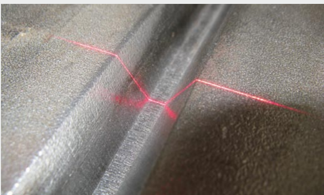
V-seam measurement on pipes
