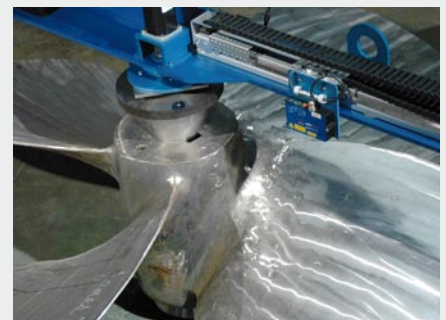
Profile measurement of marine propellers
