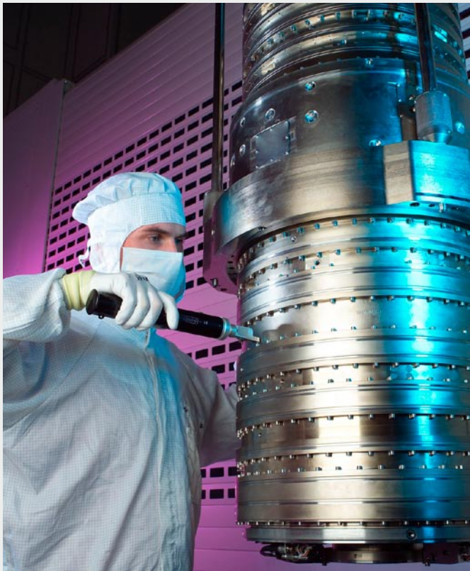
Capacitive displacement sensors are used for adjustment with nanometre precision of lenses in optical systems for wafer exposure.
