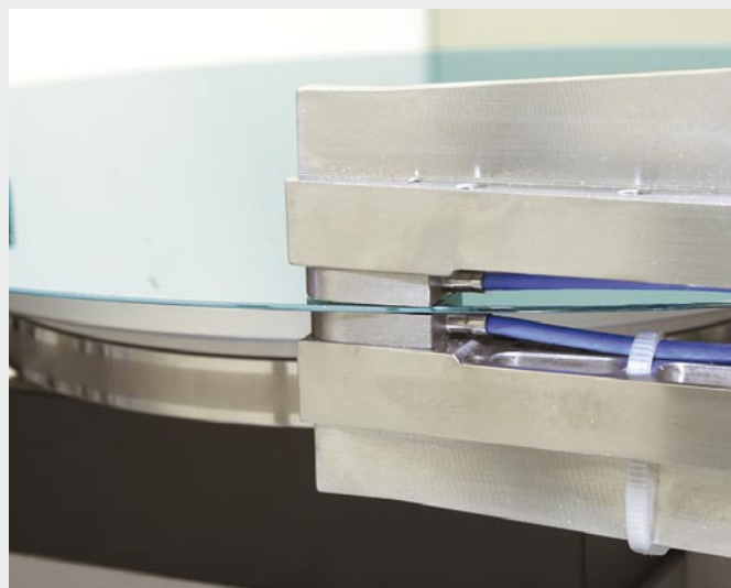
Wafer thickness measurement with two capacitive sensors
