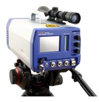
OptoMET laser Doppler vibrometers (LDV) are very fast and easy-to-operate vibration measuring instruments. They are used for precise, non-contact, and non-reactive measurements of mechanical and acoustic parameters such as vibration displacement amplitude, velocity, and acceleration.
