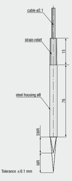
$\label{eq:MR} \begin{array}{ll} \mathsf{MR} = \mbox{Measuring Range} & \mbox{SMR} = \mbox{Start of Measuring Range} \\ \mbox{Dimensions in mm.} \end{array}$
