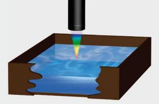
Liquid level The confocal principle enables measurements on liquids and shiny targets.
