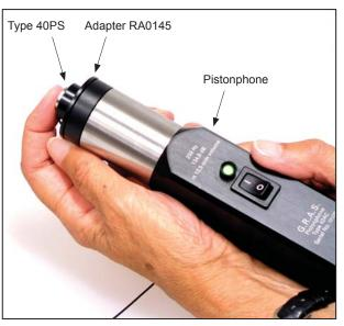
Fig. 6 Showing how the Type 40PS can be calibrated using a Pistonphone and an Adapter (both available from G.R.A.S.)
