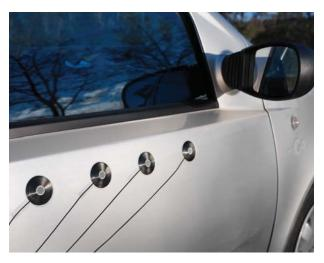
Fig. 3 An array of four Surface Microphones mounted on the external surface of a car
