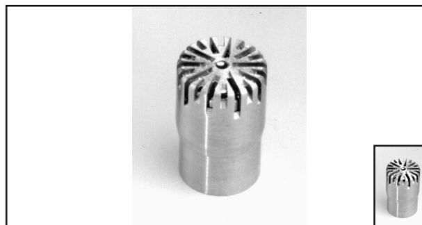
Fig. 1 1/4-inch Pressure Microphone Type 40BP (inset shows true size)
